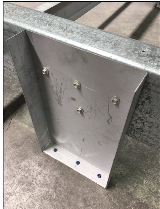
Figure 8: Mid support of test rig
