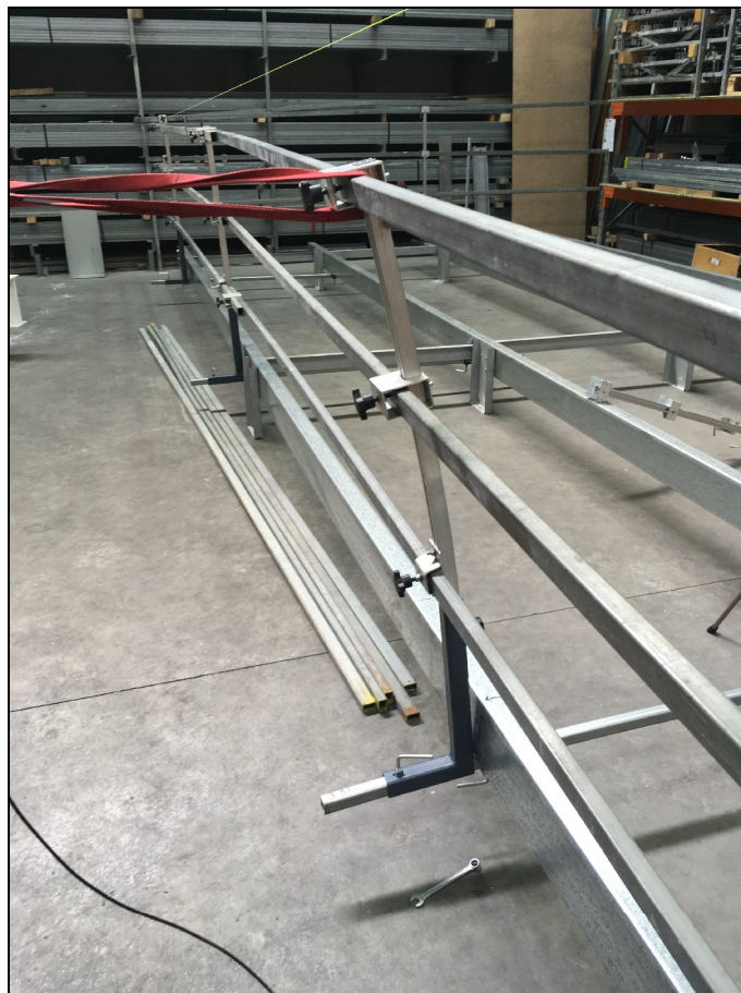
Figure 10: Post with 380 mm steel base under maximum static load
