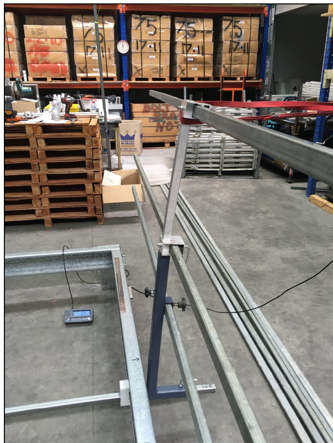
Figure 11: Post with 660 mm steel base under maximum static load
